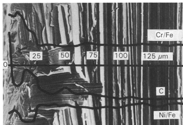
Figure 3 Profiles showing Cr:Fe, Ni:Fe ratios and the carbon content in a cross-sectional slice inside the weld bead showing enhancement in chromium and carbon near the surface (at 0 μm) of the bead.
